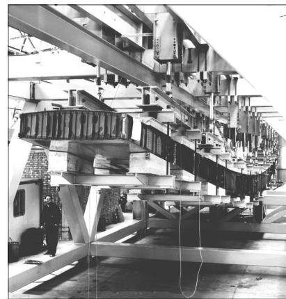
Hercules C130K Wing Fatigue Test—1979
